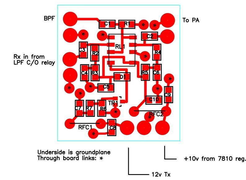
BPF switching relay using Axicom IM06 relay (Contact wetting resistors)
